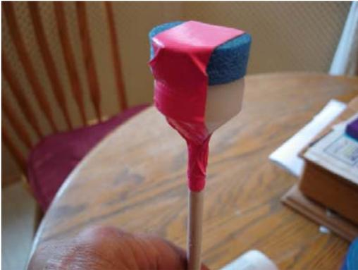
Attach the side-wrap of 1/8" closed cell foam. One or two wraps will be needed. If Lu-Shan blunts are used, one wrap will do the job as these blunts are oversized. Smaller 1.25" diameter blunts will require two wraps.
