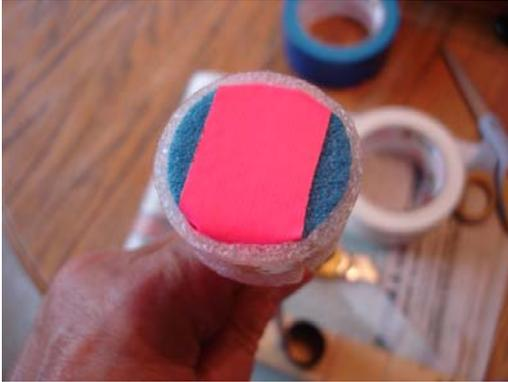
Secure the pad/blunt assembly with three strips of one-inch duck tape. Use just enough tension on the tape to force it around the corners. Do not compress the foam. The tape must extend down the shaft for at least a half an inch.
